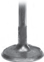
Intake Valve after P.i. Treatment
