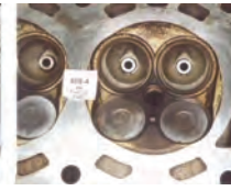
Combustion chamber after P.i. treatment.
