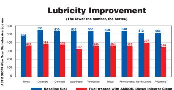
The ASTM D975 diesel fuel standard specifies a wear scar below 520 µm in ASTM D6079 testing, while the Engine Manufacturers Association (EMA) specifies a wear scar below 460 µm. Testing reveals AMSOIL Diesel Injector Clean provides significant lubricity improvement in diesel fuels found across the U.S., delivering improved wear protection.
