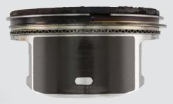
After 250 hours (13,647 miles) of dyno testing, AMSOIL 20W-50 Synthetic V-Twin Motorcycle Oil protected against piston scuffing and wear for long engine life.
